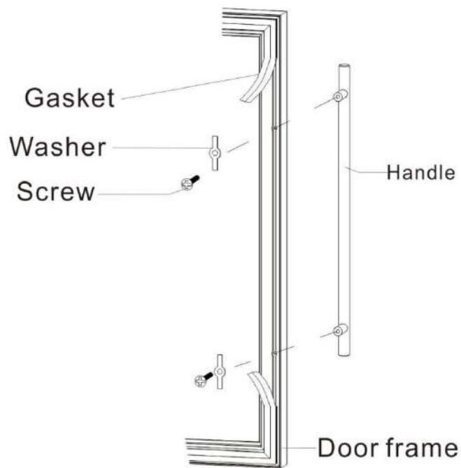
2. Align the handle with the screws and tighten the screws until the handle is both flush and secured tightly against the door frame (DO NOT over-tighten as this will cause damage to the handle assembly and door glass surface).
