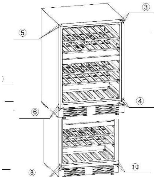
11. Turn the door by 180°, and insert the door axis into bottom door axis hole.
