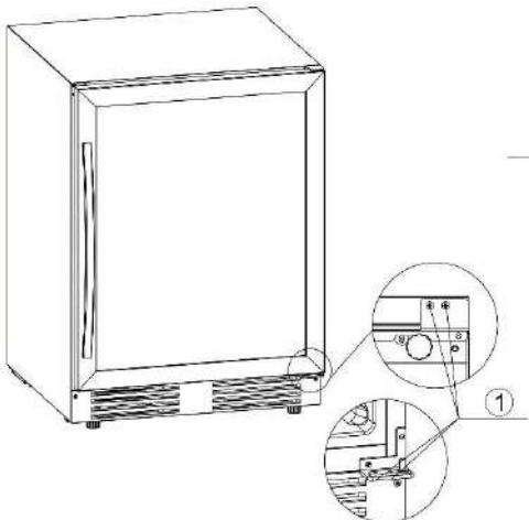
2. Remove the door axis from door axis hole at the left bottom of the door.
