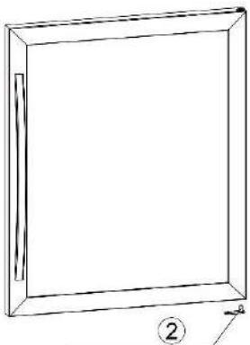
3. Remove right upper hinge by unscrewing three screws.
