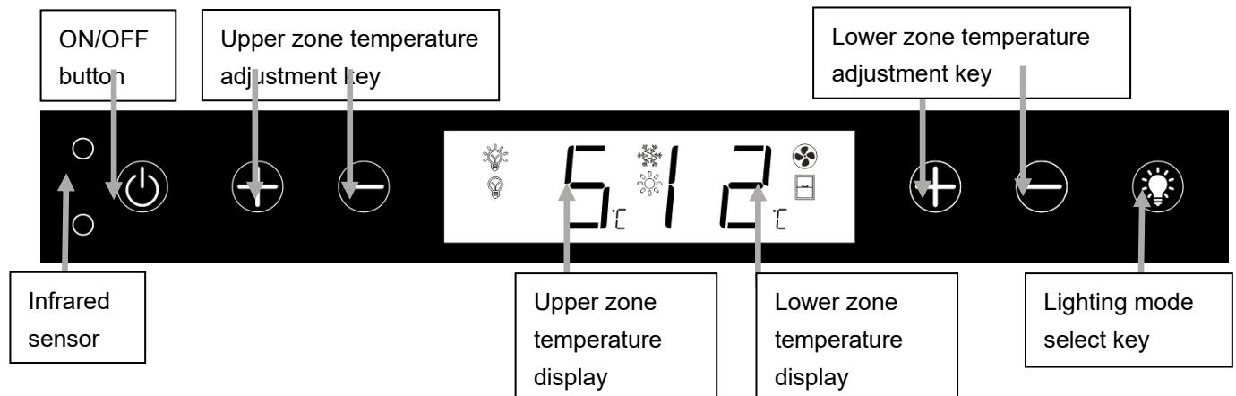
This appliance is installed with infrared sensor, to avoid malfunction of door open alarm, do not place the appliance under bright environment, or outdoor or under sunlight.
