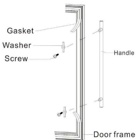
2. Align the handle with the screws and tighten the screws until the handle is both flush and secured tightly against the door frame (DO NOT over-tighten as this will cause damage to the handle assembly and door glass surface).
