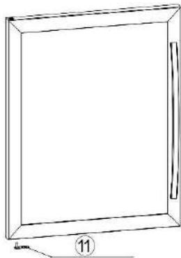
12.Put the door into left upper hinge axis, align the door with lower hinge, and fix door axis to left lower hinge.
